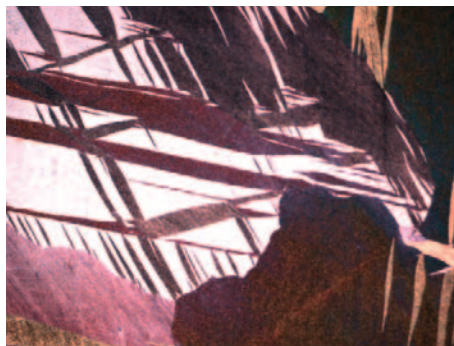
Tin with deformation twins, 1:100
