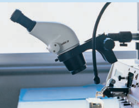
Leica S6 with 60° ergonomic viewing angle on mountable focus drive, tiltable, for OEM
